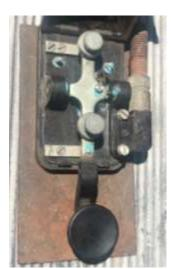
I cleaned the contacts on this Baumustuer and then attempted a CQ with my ICOM rig. It worked okay but the springs were a little strong for my taste. If I were a German tank signaller, however, and driving over rough ground, strong springs would prevent unintended keying and be a help rather than a hindrance.
